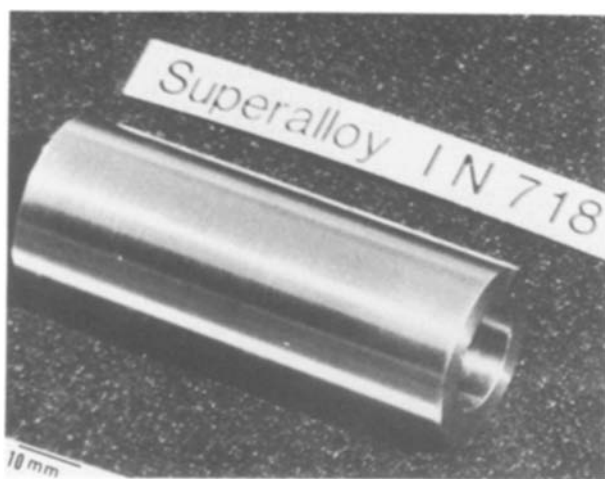
Figure 18 Photograph of specimen (Test 39) consolidated using double-tube big gap and pre-heating.
